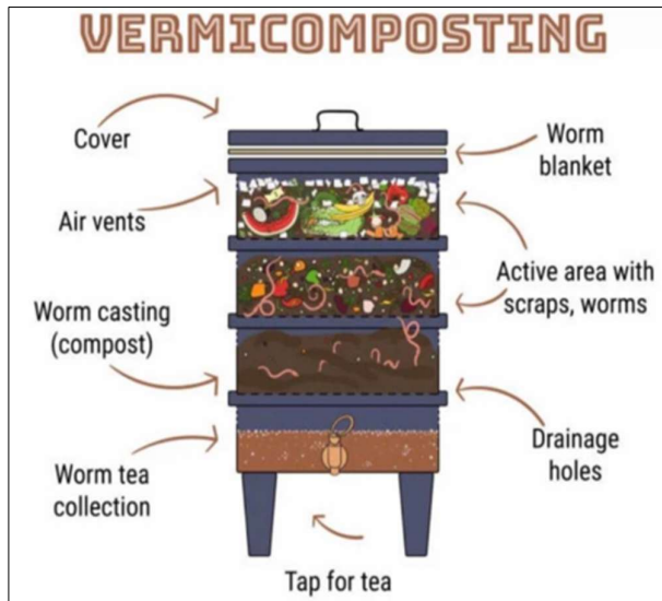
Fig 13: A diagrammatical example of a vermi-composting system.
